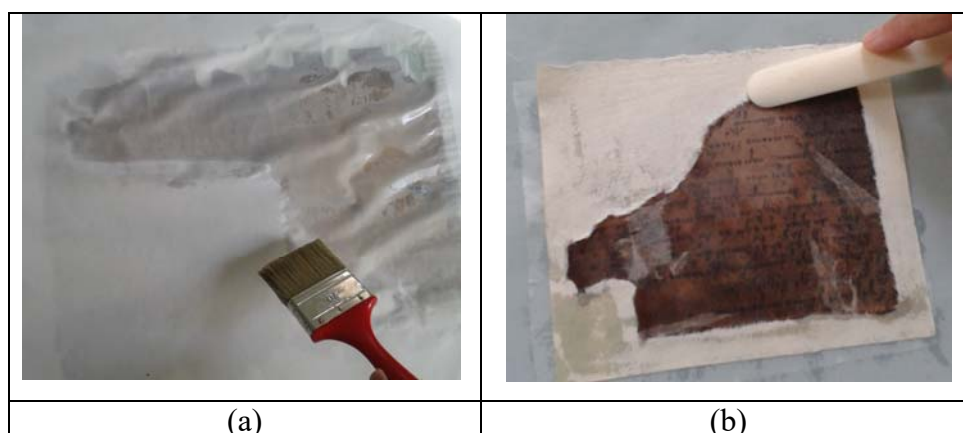
Fig. 5. Wet cleaning through the application of the compress from filter paper (a); document (1) consolidation (b)
